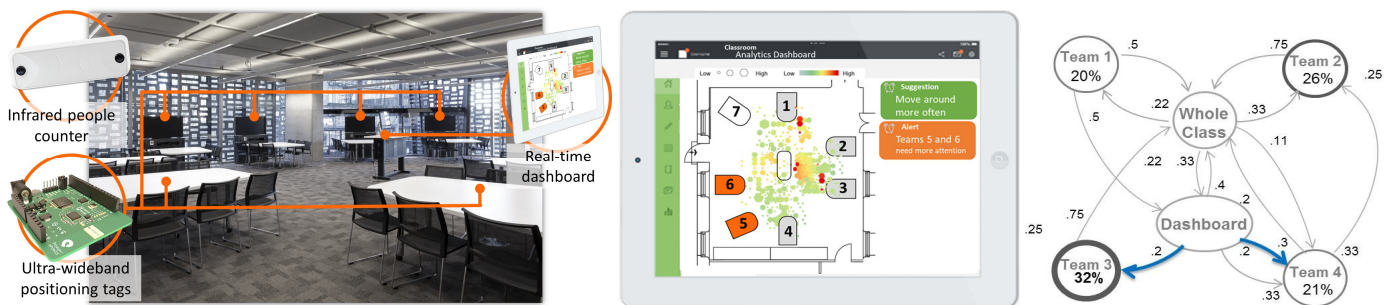
Figure 3: Left: IoT proximity/location sensors and a dashboard to be deployed in an authentic classroom. Centre: Low-fidelity prototype of a physical proximity analytics teacher’s dashboard. Right: Example of a state diagram representing the teacher’s tracked proximity data at an authentic small group classroom session.
